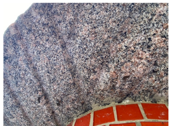
A close-up of the dressing on the millstone. Photo source: Donna Cudmore
